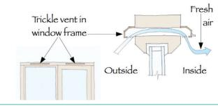
Keep the window vents (sometimes known as trickle vents) open to help air to circulate.
